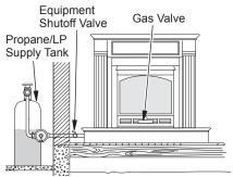
Figure 17 - Checking Gas Joints (Propane/LP Only)
